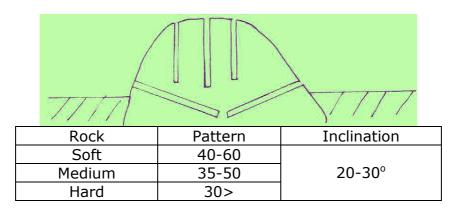
2. Breaking rock in cylindrical shape by drilling not more than 40mm diameter holes
