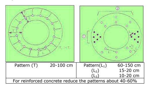
B. By drilling not more than 40 mm diameter horizontal holes
