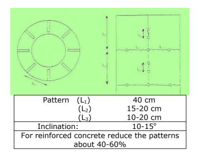
4. Breaking concrete walls and foundations by drilling not more than 40mm diameter holes.
